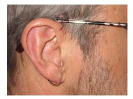
Figure 2: Binaural system for recording the sound pressure at the eardrum. The microphones are behind the pinna, with a hard tube into the ear canal, equipped with a very soft silicone tip. When high quality on-ear headphones are equalized with the same microphones and a mathematical inverse filter exceptional realism results – without the need of head tracking.
