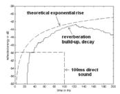
Figure 7: Reverberation build-up and decay from a 100ms excitation in a model of Boston Symphony Hall. The seat was chosen so that the D/R would be -10dB for a continuous excitation. Note that the initial delay is less than in Amsterdam. The sound is slightly less clear, but still engaging. The value of *LOC* is +4.2dB.
